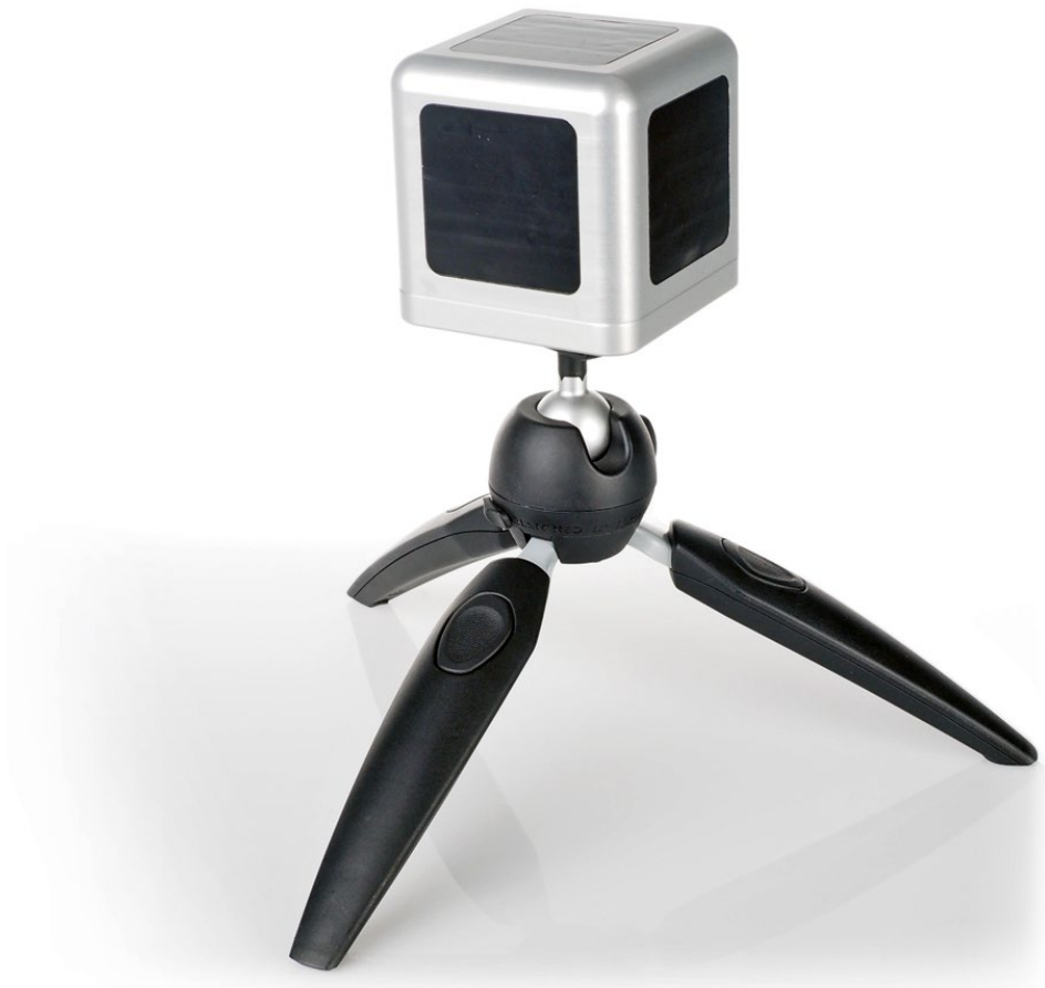
Figure 0.1 The TCOM01 sensor body on a tripod. TCOM01 is meant for surveys of thermal comfort as experienced by the human body. It is equipped with 5 x heat flux sensor (black surfaces) and a sensor body temperature sensor. Heater power, ambient temperature and relative humidity are measured in the accompanying MCU (Measurement and Control Unit)
