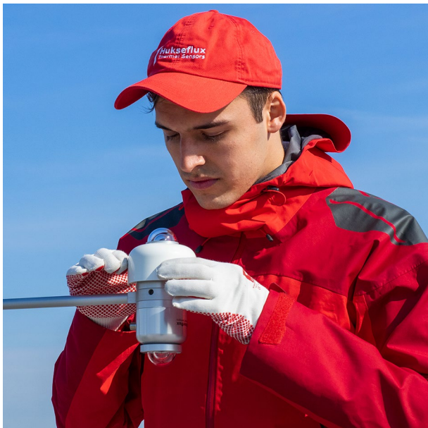
Figure 4 Using the SRA300-D1 albedometer is easy; the instrument is composed of one AMF03 and two SR300-D1 pyranometers.
