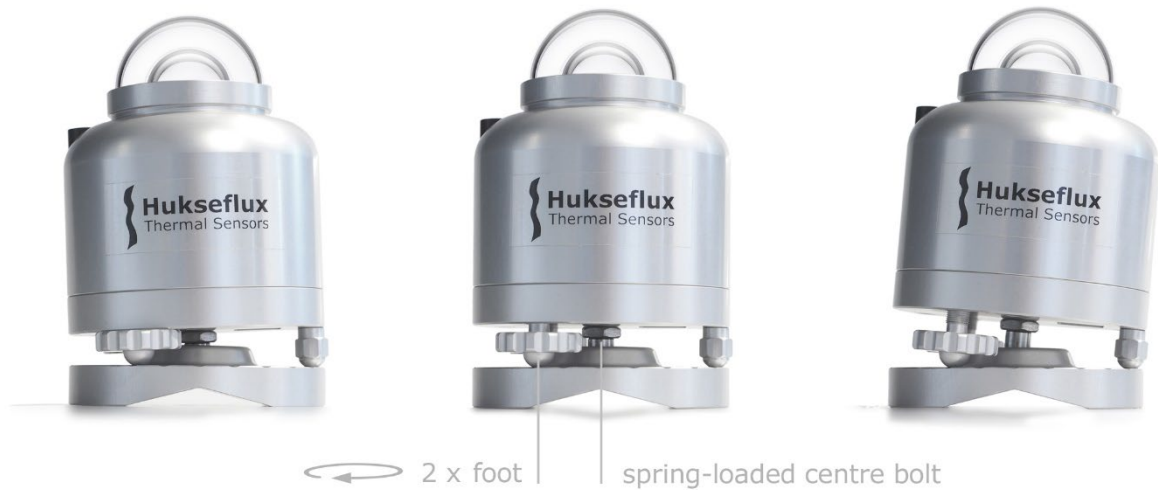
Figure 5.3.6.1.5 Pyranometer locked on its optional levelling mount: by fastening (on the left) or loosening (on the right) the two adjustable feet, the pyranometer can be levelled, using the bubble level as a reference. The static foot remains fixed. In all cases, ensure the legs of the pyranometer fit into one of the small ledges of the levelling mount. Locking is in place, when the nut is turned all the way against the bottom plate of the pyranometer.
