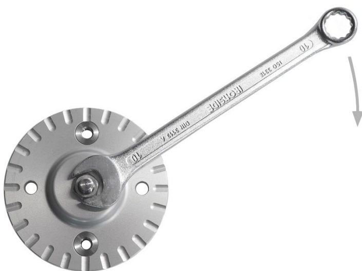
Figure 5.3.6.1.3 LM01 levelling mount seen from above: (un)locking with a 10 mm spanner.
