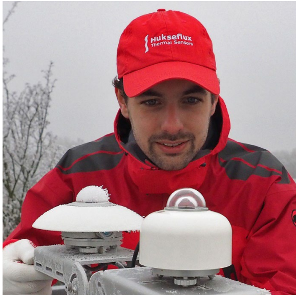
Figure 0.5 SR300-D1 is heated to counter frost and dew deposition: clear difference between a non-heated pyranometer (back) and a heated pyranometer (front).
