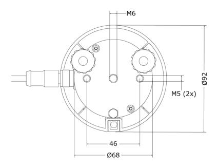
**Figure 3.5.2** Dimensions of Hukseflux industrial pyranometers.
