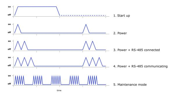
Figure 6.2.1: Power and communication status LED behaviour
