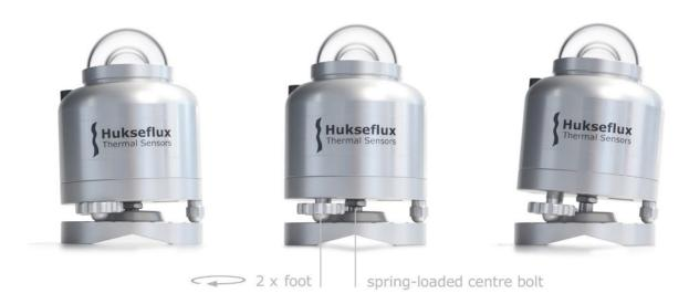
**Figure 0.9** LM01 levelling mount is the most popular option for pyranometers: practical spring-loaded mount for easy mounting, levelling and instrument exchange on flat surfaces. The spring-loaded mounting has the advantage that levelling can be done quickly, without unlocking the instrument.
