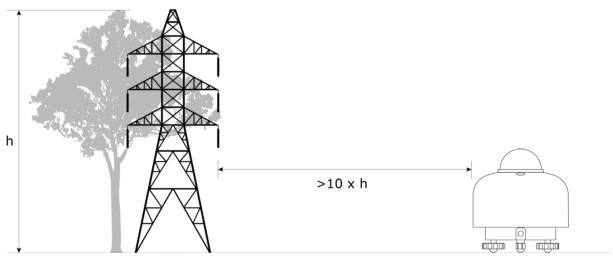
**Figure 5.1.1:** Preferably, the field of view of the pyranometer should be unobstructed by nearby obstacles. If obstructions are present, as a rule of thumb the pyranometer should be installed at least 10 times the height of the obstruction away from the obstruction.
