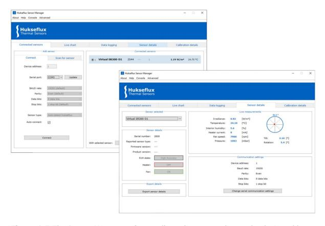
**Figure 0.7** The Sensor Manager software allows the user to change the device address and communication settings.
