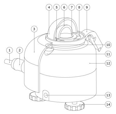
**Figure 3.5.1** *Hukseflux industrial pyranometers components*:
