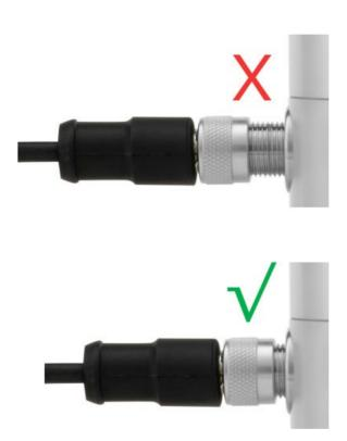
**Figure 5.3.4.1** Connection of the cable connector to the chassis connector: make sure to completely tighten the screw lock. This is necessary for proper sealing against moisture and proper electrical connection of conductors and cable shield.
