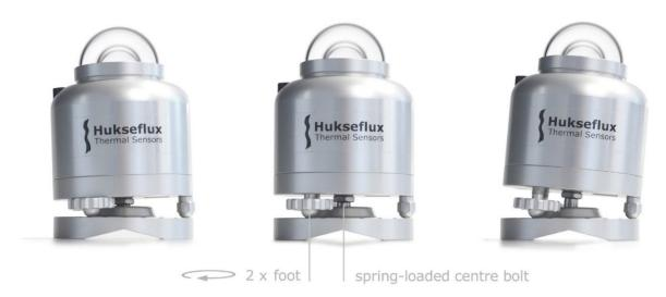
**Figure 5.3.6.1.5** *Pyranometer locked on its optional levelling mount: by fastening (on the left) or loosening (on the right) the two adjustable feet, the pyranometer can be levelled, using the bubble level as a reference. The static foot remains fixed. In all cases, ensure the legs of the pyranometer fit into one of the small ledges of the levelling mount. Locking is in place, when the nut is turned all the way against the bottom plate of the pyranometer.*
