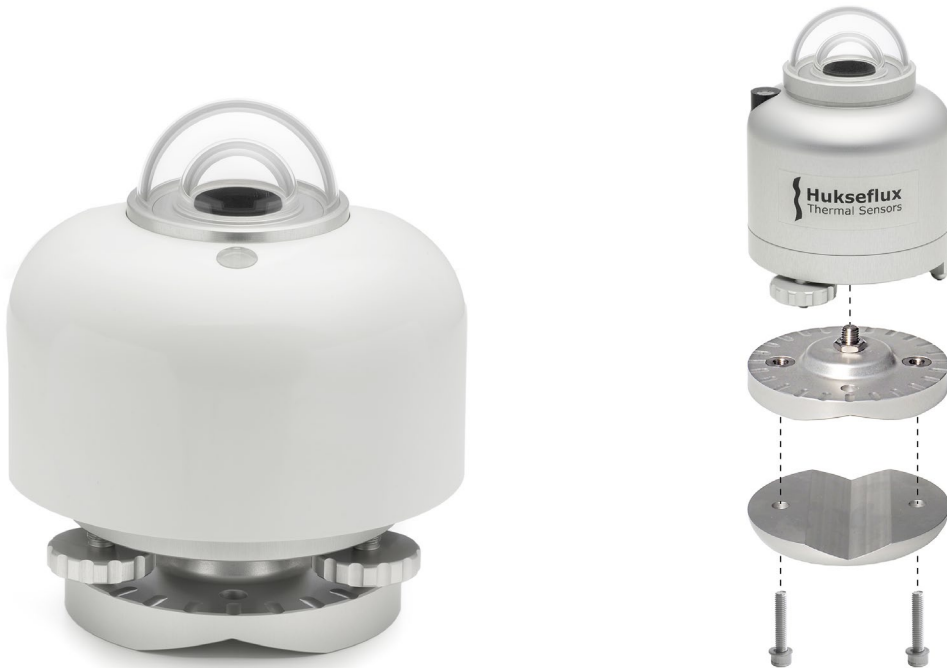
Figure 0.2 Optional levelling mount (picture on the left); a practical spring-loaded mount for easy mounting, levelling and instrument exchange on flat surfaces, and the optional tube mount (picture on the right) including spring-loaded levelling upper clamp, lower clamp for tube mounting and two sets of bolts.
