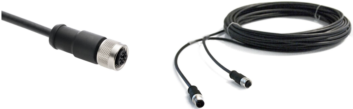
Figure 0.4 On the left the SR15-A1 cable with M12-A female connector on sensor end, stripped over 0.15 m and conductors with ferrules. Its length is 5 metres standard and available in 10 and 20 metres too. On the right the optional Hukseflux extension cable with connector pairs, with male and female M12-A connectors, available in 20 metres
