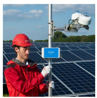
**Figure 1** Surge protection upgraded to Level 4. One SPD01 Surge Protection Device can protect up to 3 pyranometers.
