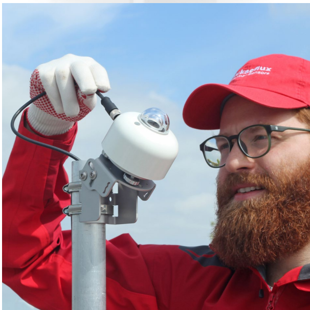
Figure 2 PMF01 pyranometer mounting fixture can be used for easy installation of a pyranometer, in this case SR30-M2-D1, in Plane of Array for PV system performance monitoring and meteorological applications.
