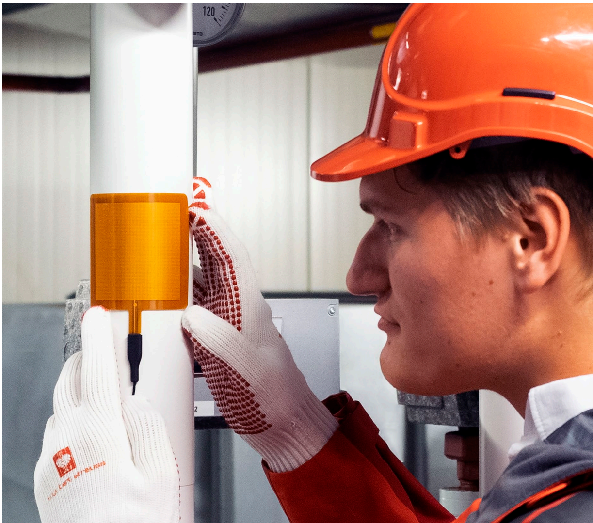
Figure 4.1.1 Example of model FHF05-85X85 foil heat flux sensor being installed for measurement on an industrial pipe. The sensor is mounted on a well-prepared curved surface.
