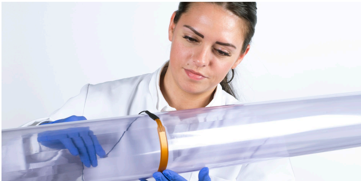
Figure 0.2 Model FHF05-15X85 foil heat flux sensor being installed to measure heat flux on a pipe.
