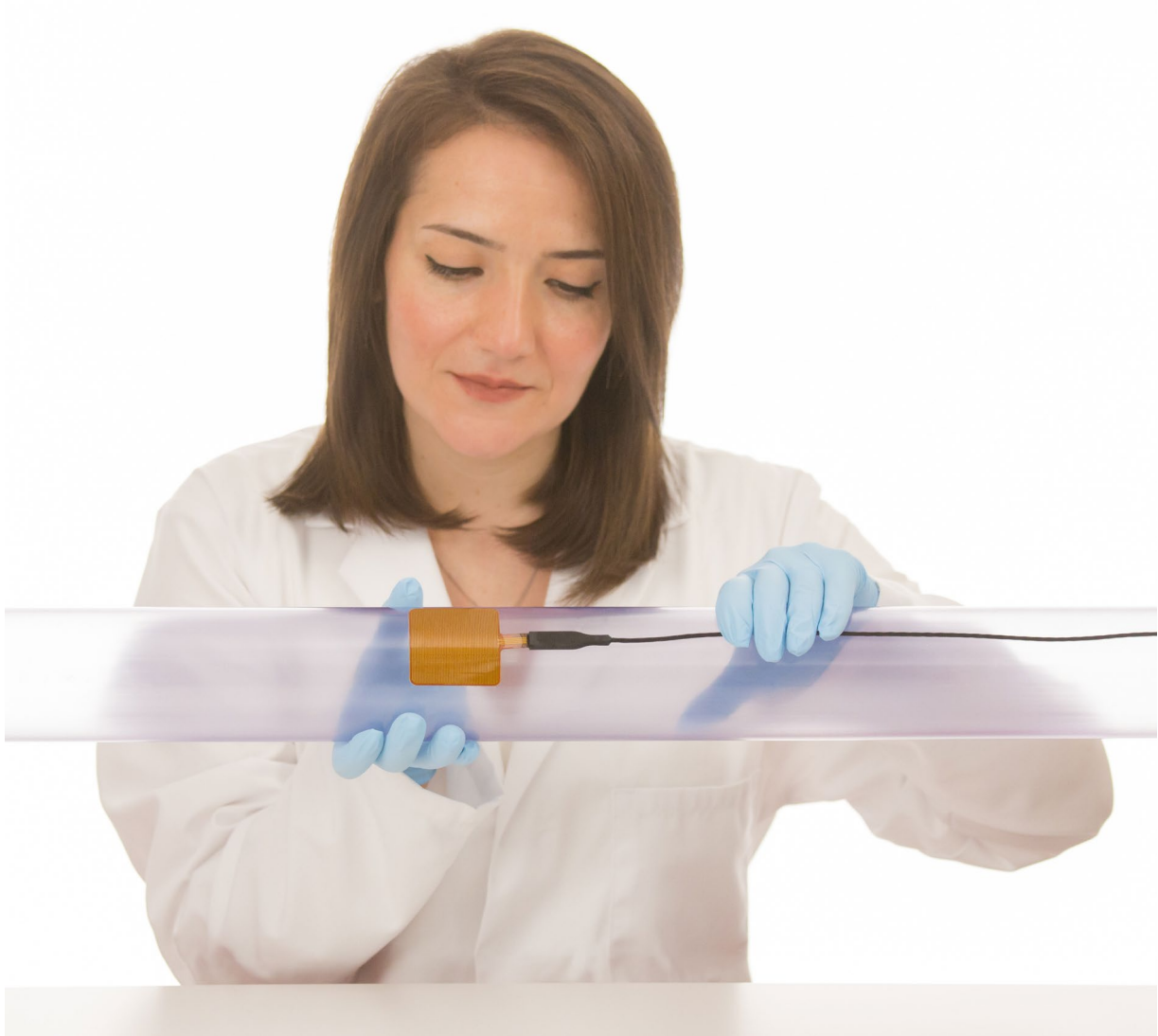
Figure 0.2 Application example: FHF05SC-50X50 is being installed to measure heat flux on a pipe. The sensor is mounted on a well-prepared curved surface.
