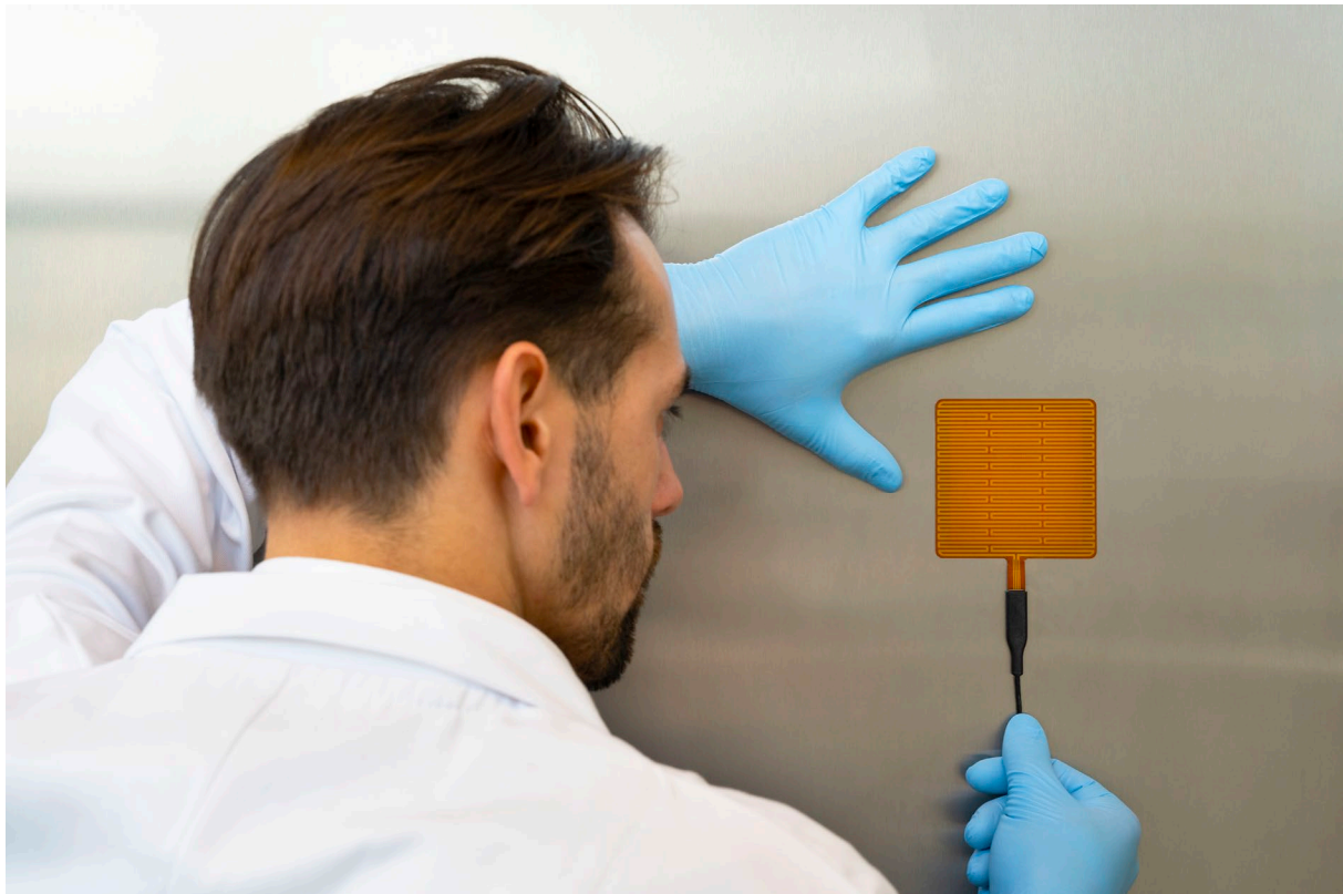
Figure 4.1.1 Example of model FHF05SC-85X85 foil heat flux sensor being installed for measurement on an object. The sensor is mounted on a well-prepared flat surface.
