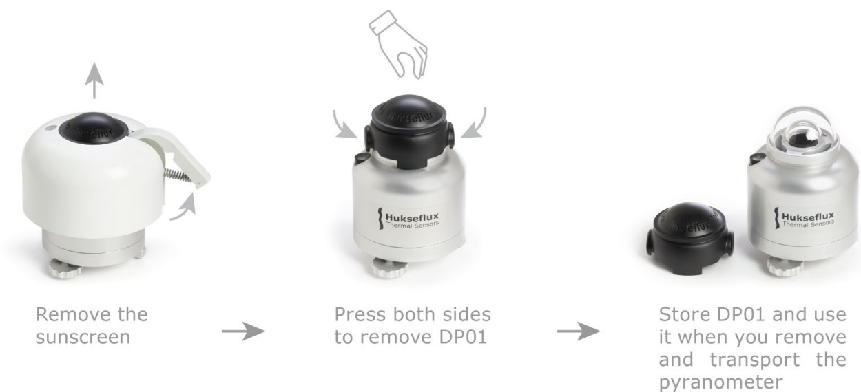
Figure 2 Removal of the sunscreen and DP01.
