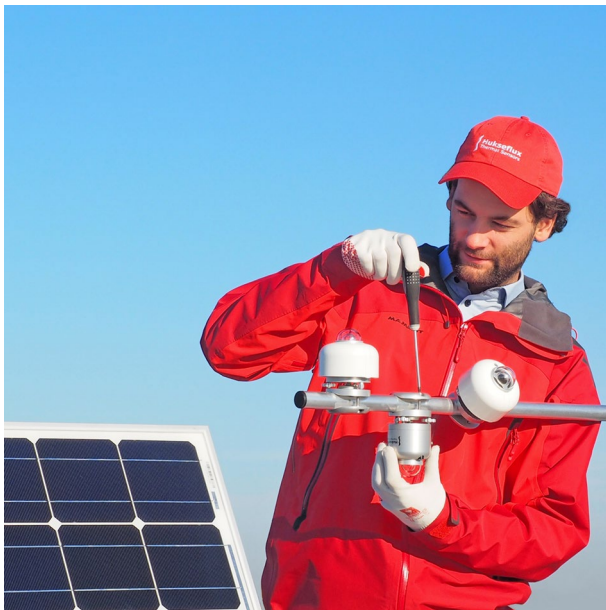
Figure 2 A crossarm can be used for easy installation of a pyranometer, in this case SR30-M2-D1, in Plane of Array, horizontal or inverted for PV system performance monitoring.
