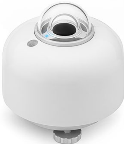
Figure 2 Example of a Hukseflux spectrally flat Class A pyranometer, model SR300-D1. This model is recommended for PV system performance monitoring as well as research-grade diffuse radiation measurement. Digital output via Modbus RTU over RS-485.
