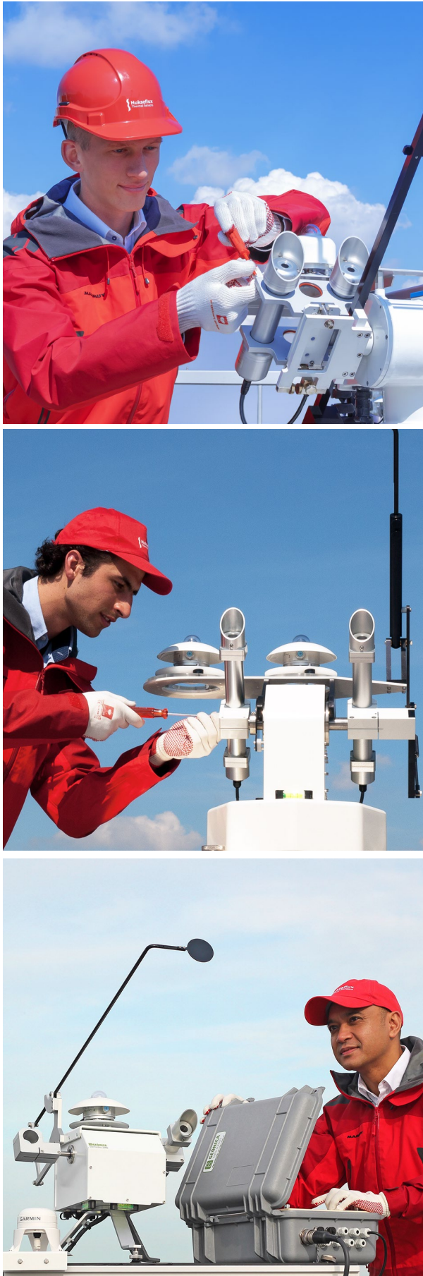
Figure 6 Pyrheliometers mounted on solar trackers.
