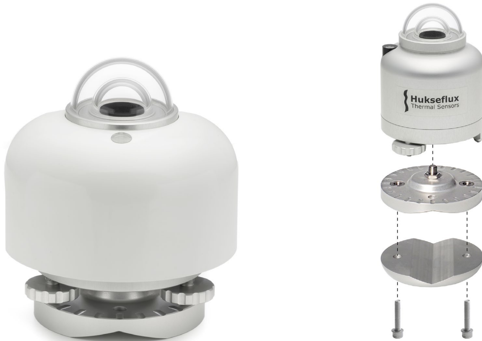
Figure 0.3 Optional levelling mount (picture on the left); a practical spring-loaded mount for easy mounting, levelling and instrument exchange on flat surfaces, and the optional tube mount (picture on the right) including spring-loaded levelling upper clamp, lower clamp for tube mounting and two sets of bolts
