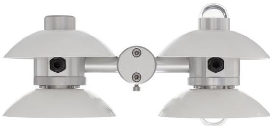
**Figure 1** NR01 4-component net radiometer, including two pyranometers, two pyrgometers, a heater and a 2-axis levelling assembly
