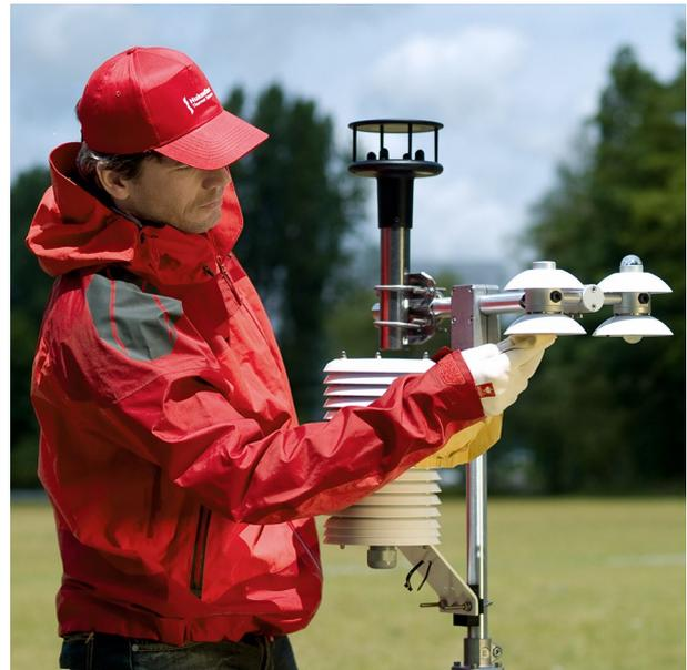
**Figure 2** NR01 4-component net radiometer in use in a typical meteorological station
